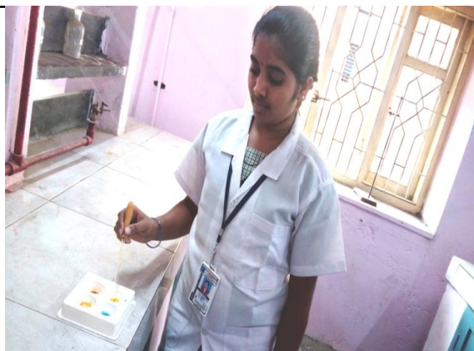
Student performing qualitative tests for ions over a spot test plate.
